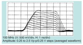
Variable level (amplitude) characteristics
