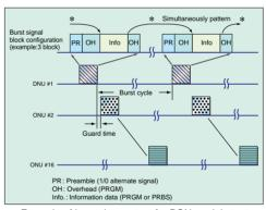
Example of burst data output for PON module test
