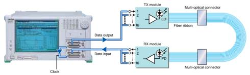
Testing example for optical multi-channelmodule
